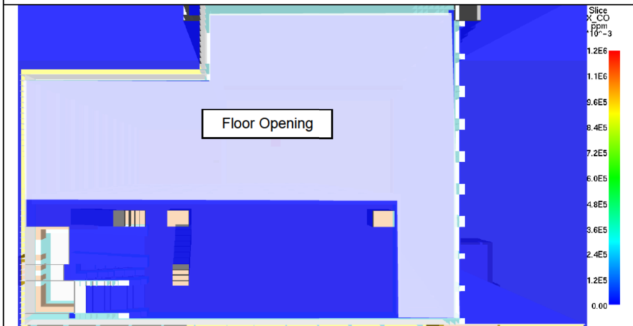
Figure 3: CO Concentration 6 Feet above Floor 17 Design Fire 1 Trash Can Fire under Floor Openings
