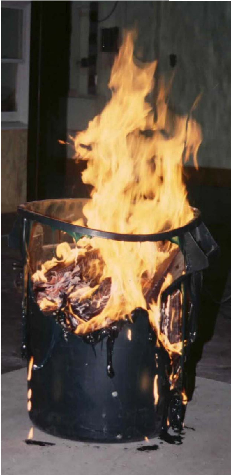
Figure 6. Fire continues to grow in Trash Container 1.
