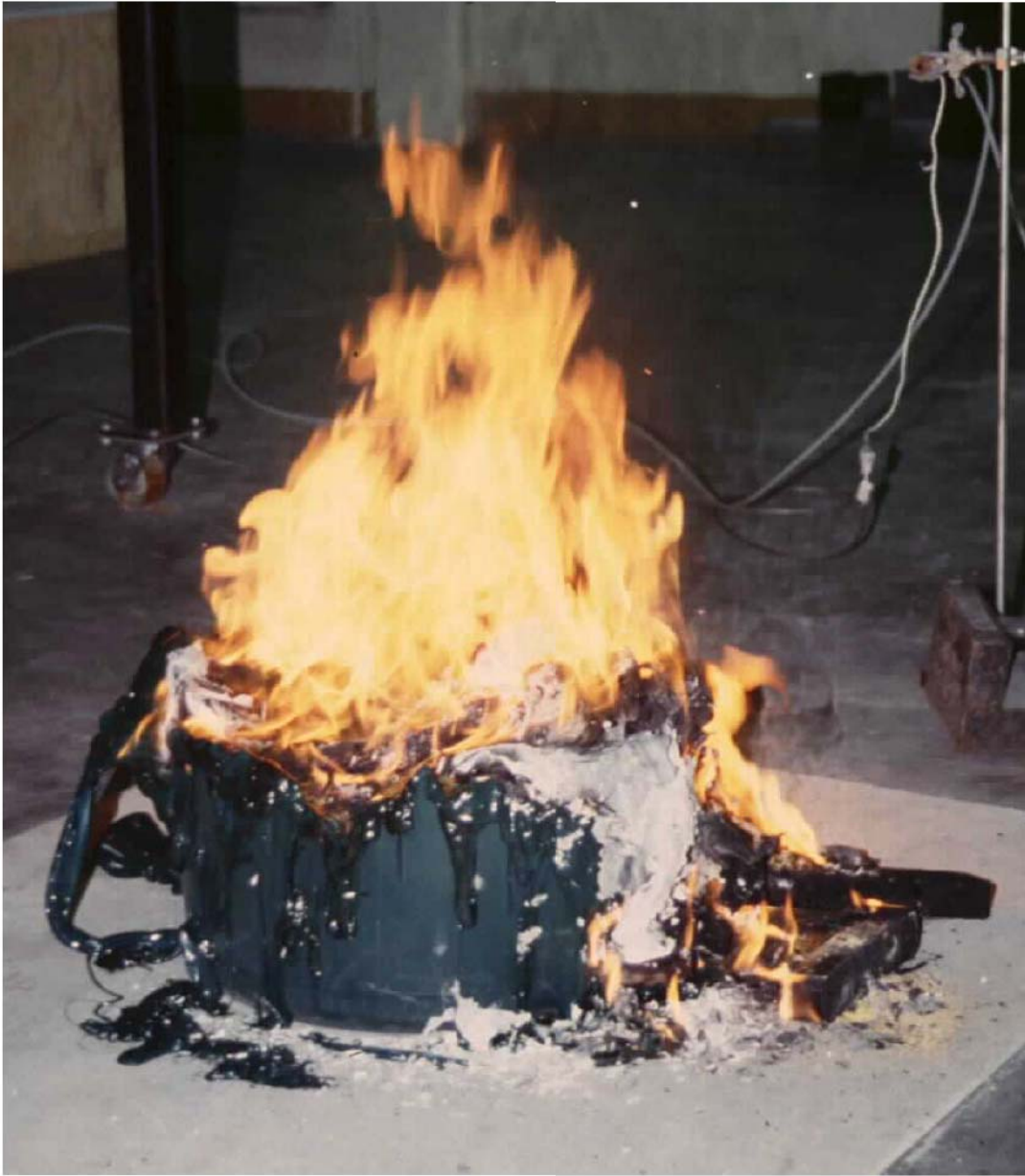
Figure 7. Upper portion of container melts and collapses.
