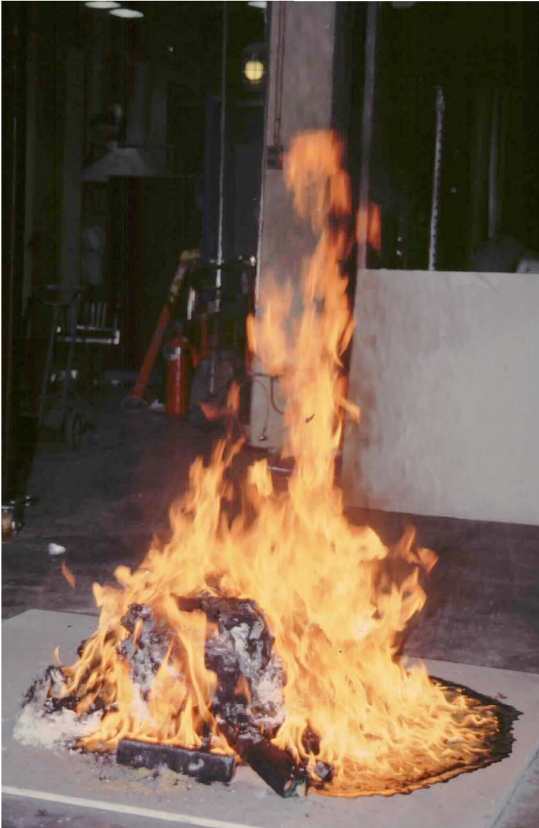
Figure 8. Molten plastic burning around debris pile.
